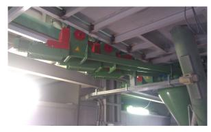
To prevent influences through wind, the new weighing scale was placed inside a protective housing. For the dosing, we chose special screws with a very small "drop". This produces still higher product quality and less spillage of extremely expensive raw materials. The extension in the number of automated dosages has strongly reduced the number of manual dosages. This efficiency improvement is helping **OMNICOL** to keep producing its high-quality products for the building world.
